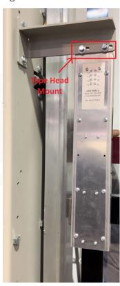
Once the bracket for the tape head is installed, mount the tape head in the two slotted holes of the bracket using the provided hardware, as shown in Figure 18.
